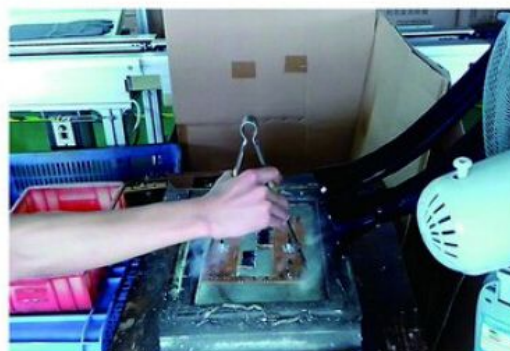
Tin soldering supported fume extraction
